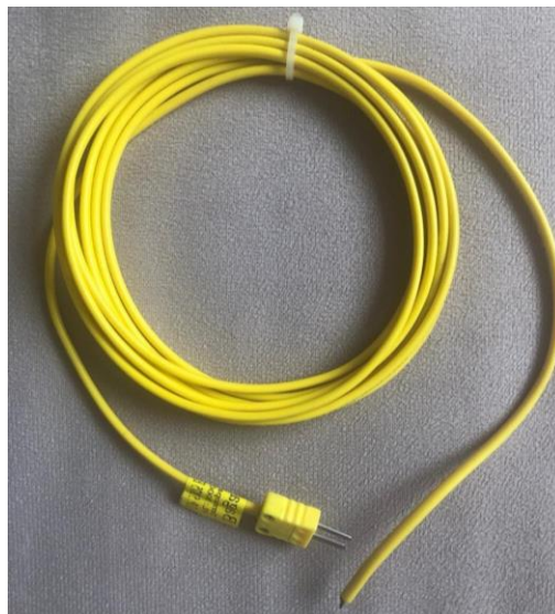
Figure 12 - Thermocouple for monitoring the temperature inside the foundation block
