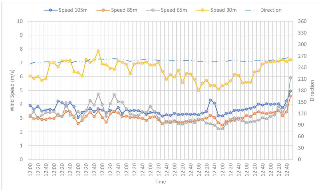
Figure 4 The influence of 2# Wind Turbine on Met Mast
