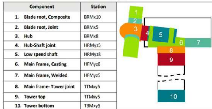
Figure 4 Critical wind turbine parts considered
